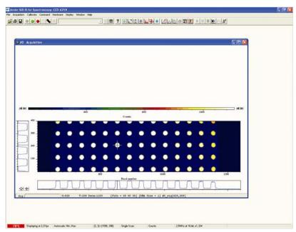
The cross-hair (see also Large Cursor and Show 2D Cross Sections under Preferences later in this section) moves to any point on the image that you click. The data value for the point, along with the pixel numbers on the x- and y-axes that identify the point, is displayed on the bottom edge of the data window.
