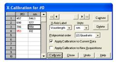
From Pixel 706 to Pixel 953 the user has indicated a fall in wavelength, despite the preceding rise in pixel 690. In such a case, an illegal non-monotonic calibration (as shown on the graph below) results.
