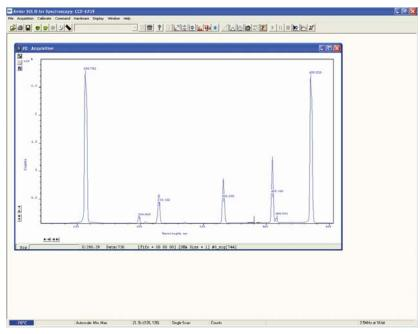
When labeling is selected, you can label a peak manually by double clicking it. To remove a peak label, double click it again. If you switch off peak labeling, (by clicking the button), your manual labeling will be lost.
