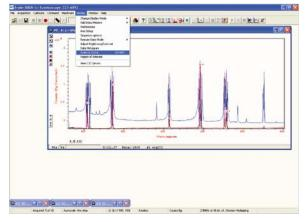
When Scale to Active is selected, all the data traces in your data window will be plotted against the scales of the active trace, e.g. for the red trace:
