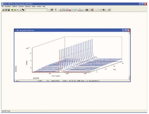
Along with the x-axis (calibrated by default to represent pixels across the CCD-chip) and the data-axis (calibrated by default in counts), you now see a 3<sup>rd</sup> (or y-axis) calibrated in rows or tracks, depending on the acquisition mode you have selected.
