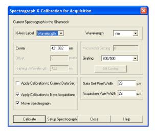
NOTE: The dialog box can also be opened by selecting the Setup Spectrograph option from the Hardware menu on the main window.
