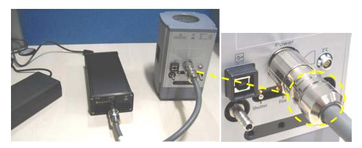
Figure 5: PS30 connected via Power Cable PS40 to camera
