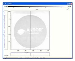
The scale on the Palette bar is calibrated in your chosen data units. By default, the full range of colors/grays is correlated with the full range of data in your data set. This is known as 'Rescaling' (see Rescale on page 108).
