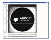
The arrow buttons at either end of the palette bar can be used to adjust the manner in which values are mapped against colors, and so change the brightness and contrast of the image. See next page for further details of the Pallete Bar.
