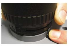
Press the catch down, screw the lens in carefully counter-clockwise and it will then lock into position
