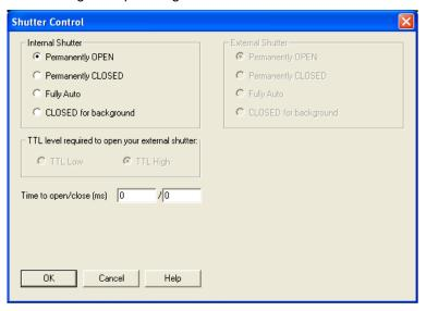
You can use this to indicate when and how a hardware shutter should be used. With a CCD, the shutter is used for background shuttering. Certain settings (e.g. **Permanently OPEN & Permanently CLOSED)** take effect as soon as you close the Shutter Control dialog box. Other settings will be applied whenever you acquire data.
