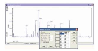
The user can now enter and define customized baselines. The values to be subtracted are entered against individual pixel numbers in the dialog box. The user can select whether to fit the data using polynomial or cubic spline. The user can also select where the **Corrected** and **Baseline** data are stored. When the necessary parameters have been set and the **Apply** button is clicked, other data windows will be generated as defined by the user, e.g.:
