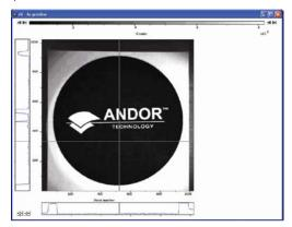
• The arrows to the right of the Palette bar on the Data Window allow you to adjust the maximum distinguishable data value (i.e. max, the value at which the Palette Bar becomes white), e.g.:
