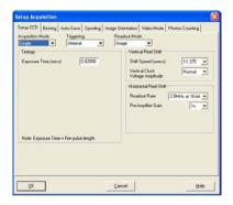
**Single** scan is the simplest acquisition mode, in which the system performs one scan of the CCD.
