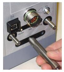
Figure 8: Fitting a mounting post
