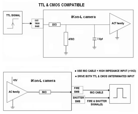
NOTE: The shutter pulse is fed from the Shutter SMB on the back of the camera.
