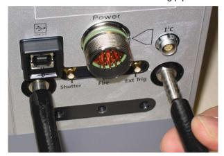
These can be connected to a water cooler or recirculator to improve cooling.
