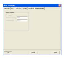
**Photon Counting** is a technique used to record very low-level signals that might otherwise be lost in background noise.
