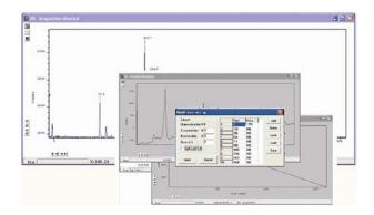
Window #0 will show the raw data as acquired during the last acquisition, by default window #2 will show the profile of the customized baseline to be subtracted off the raw data and window #1 will show the baseline corrected data i.e. #0 - #2). The window number labels of the customized baseline profile and corrected data can be adjusted by changing the numbers detailed in the Baseline correcting dialog box.
