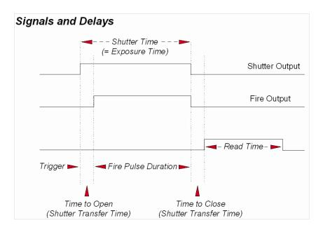
If you do not have a shutter connected, set the Time to open or close to 0. Setting the Time to open or close to any other value will insert extra delays into cycle time calculations.
